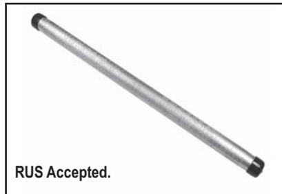
Single-sleeve aluminum UNISPLICE™ designed to splice ACSR as simply as all aluminum. Pre-filled with PENETROX™ joint compound, stripsealed and capped to limit oxide growth and to increase the life of the connection. Eliminates strand stripping, installing separate steel sleeve
