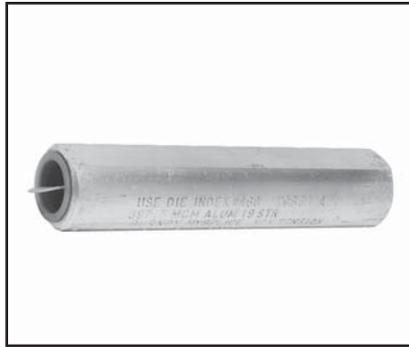
Full-Tension HYSPlice™ sleeve made of aluminum tubing with staked-in cable stop. Sizes 1/0 and larger tapered for gradual transition of stress. Installed with HYSPlice™ tools and
