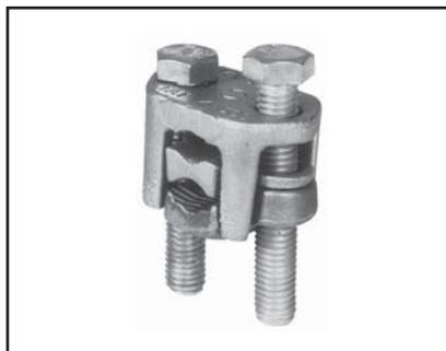
Similar to OKLIP™ Type KVS except for a high copper alloy spacer that separates run and tap conductors. Provides high contact pressure, confines conductor strands, and assures vibration-proof connection. Longer peened bolt, permits swivel action for easier installation. Silicon bronze DURIMUM™ hardware.
