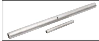
Full tension, two-piece, compression splice for ACSR transmission lines up to and including 230 kV. Outer aluminum sleeve has filler hole and plug for PENETROX™ joint compound. Kit includes the outer aluminum and inner steel sleeve.
