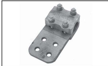
Aluminum alloy bolted type terminal for joining aluminum tube to copper or aluminum pads. Drilling in pad conforms to NEMA Standards. PENETROX™ joint compound recommended on contact surfaces.
