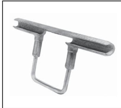
Permanent compression hot-line clamp adapter with aluminum run and copper bail. Accommodates any standard copper hotline clamp on bail elements. Permits hot-line tapping without arcing or chafing damage to aluminum conductor. Installed with standard tools and dies. Prefilled with PENETROX™ joint compound and stripsealed to limit oxide growth and to increase the life of the connection.
