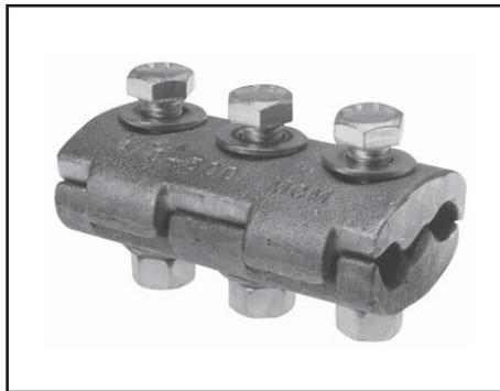
Type CP-A is recommended for tap or parallel connections. High strength, high conductivity aluminum body and hardware provide corrosion resistant assembly. Long contact surface insures excellent contact and full conductivity. PENETROX™ joint compound recommended for all combinations.
