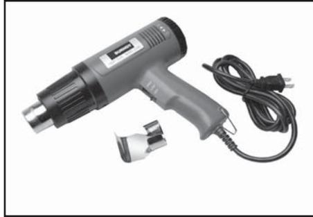
Multi-purpose, low cost heat gun has an electronic variable thermal control dial. BHS1100 meets the requirements of UL. It has a temperature range of 250° - 1100° F (121° - 650° C). 2 speed motor. Built-in safety stand heat guard included. Professional heat gun and accessories are recommended for all of your BURNDY heat shrink applications.
