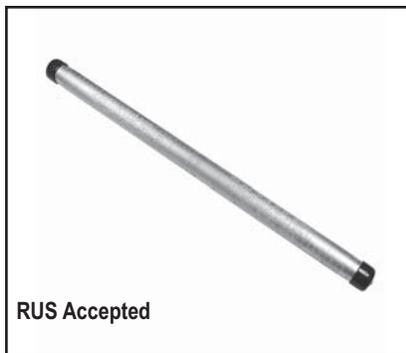
Single-sleeve aluminum UNISPLICE™ designed to splice ACSR as simply as all aluminum. Pre-filled with PENETROX™ joint compound, stripsealed and capped to limit oxide growth and to increase the life of the connection. Eliminates strand stripping, installing separate steel sleeve
