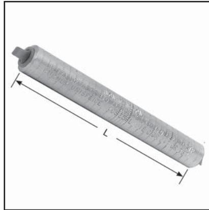
Aluminum jumper sleeve, with cable stop, designed to be installed with same dies as equivalent full-tension UNISPLICE™. Withstands jumper loop-tension and vibration stresses. Pre-filled with PENETROX™ joint compound, stripsealed and capped to limit oxide growth and to increase the life of the connection.
