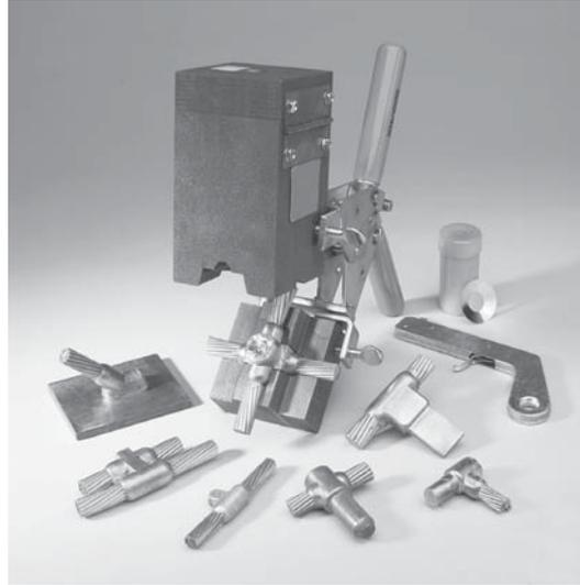
This system is very field friendly, since it is light and portable and requires no outside power source. It requires very little time or skill to obtain an efficient, maintenance free connection when using the BURNDYWeld® process.
