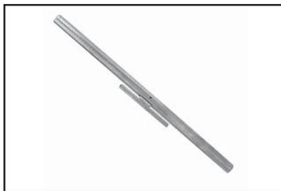
Two-piece, full-tension HYSPLICE™, made of aluminum outer sleeve and steel sleeve for steel core. Designed to be installed with BURNDY® EEI dies. BURNDY® and EEI die index numbers are clearly marked on the sleeve.
