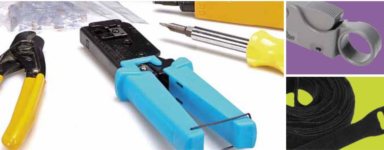
Leviton has everything you need to terminate and connect audio, video and network wiring in the home. The Wire Punchdown Tool enables one-step punchdown of 110-Style or 66 Connecting Block IDCs with a single push on the handle. Specialized blades, stripping and crimping tools, and other accessories complete the collection.
