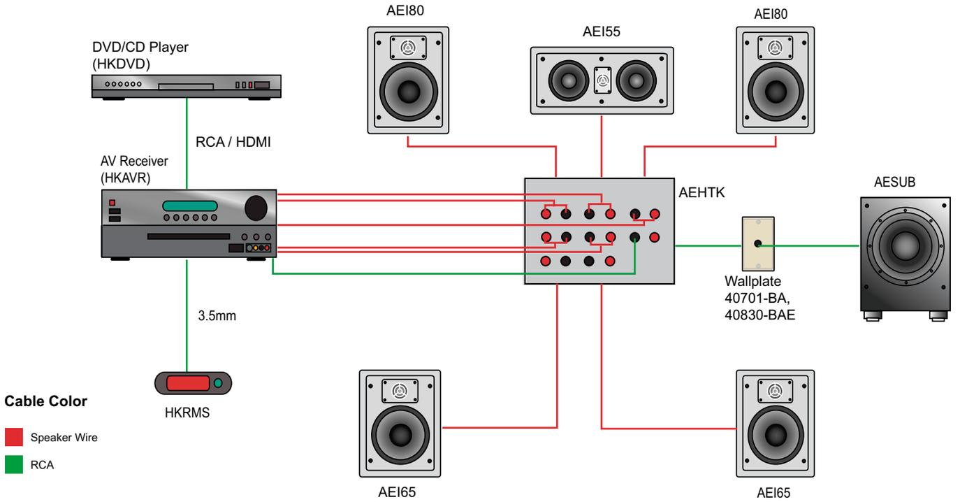
Adding a Single Source/Multi-Room Audio System to an A-BUS® Ready Audio/Video Receiver (AVR)
