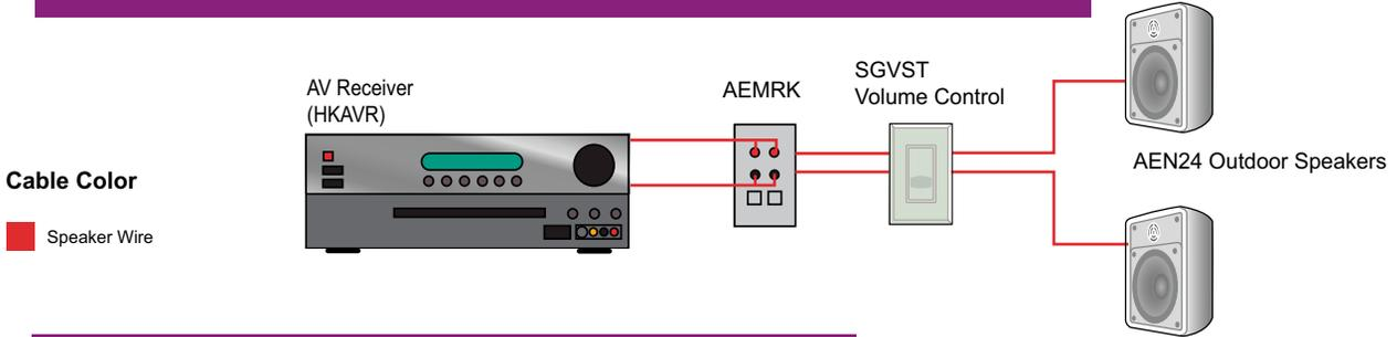
**Multi-Room Audio System Using System Matching Module**
