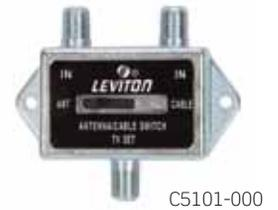
Three 75 Ohm inputs can be used for cable in, antenna in, VCR in, or any combination. One 75 Ohm connection out. Select one of three signals to be viewed.
