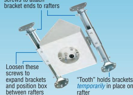
Loosen these screws to expand brackets and position box between rafters
