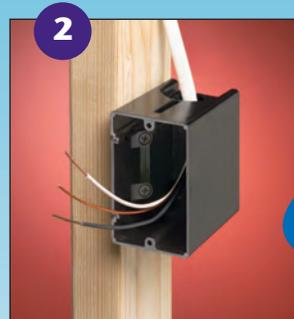
2 Pull wire through the knockout connector. (Ships with installed NM cable connector.)
