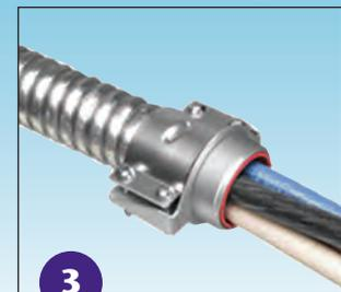
**3** No need to remove strap – simply loosen the screws and insert end stop bushing, if necessary. Slip connector onto MC cable. Retighten screws on strap.
