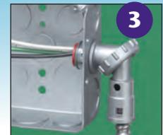
3 Tighten nut. Snap assembly into the KO.
