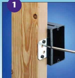
1 Attach IN/OUT BOX to wood or steel stud with captive installation screws. Feed the wires through the knockout.
