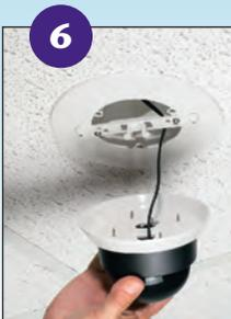
6 With camera mounted, install the mounting plate to the box by placing it on the bracket and turning clockwise to lock. Install set screw.
