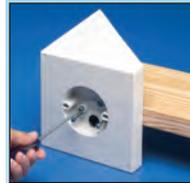
Install the FB450 on the 2x8 using the (2) #8 x 1-1/2" long parked screws provided.
