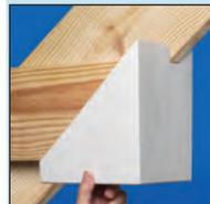
Score and trim the FB450 as necessary, keeping bottom of box level. (Short side needs to touch rafter.) Trim wood as necessary to butt it to rafter. Nail or screw assembly to rafter.
