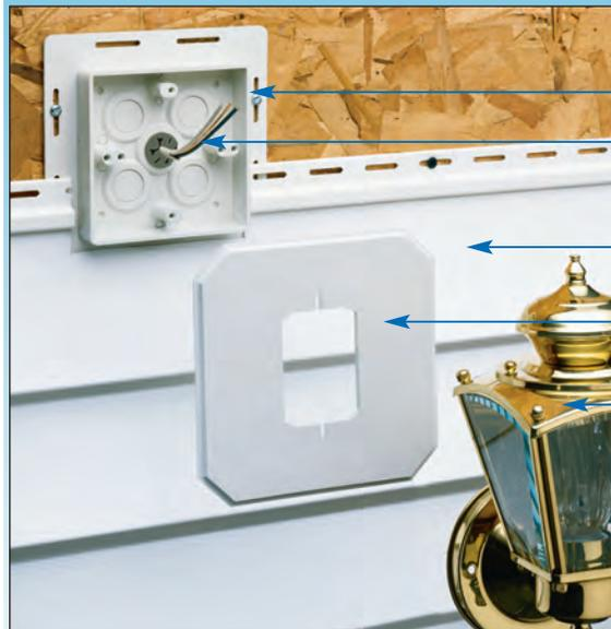
1. Before siding is installed, using the flanged style, screw the box to the wall using the holes provided in the flange.
