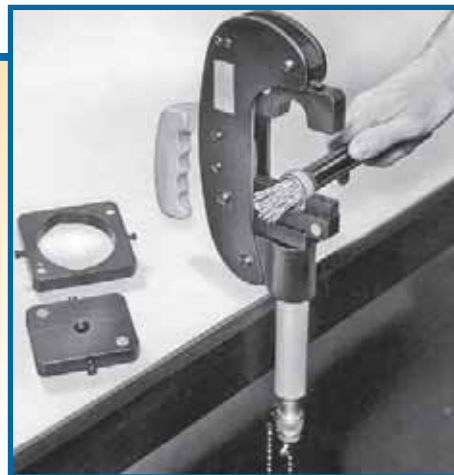
All the two-piece Shield-Kon® in the circular range need to be crimped with the 13640 hydraulic head equipped with the appropriate die.
