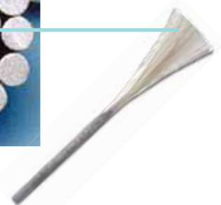
Closeup of 3M ACCR core material, consisting of aluminum oxide fibers embedded in high-purity aluminum.
