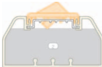
Wirefill #2: TG-70 with Data Only using "Snap-On" Faceplates and Wire Retainer
