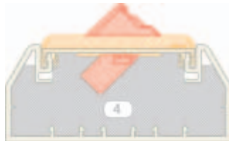
Wirefill #4: Data Only using Horizontal Sloped "Snap-On" Communication Faceplates
