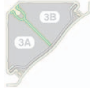
Wirefill #3: Divided Channel (Power and Data) with Wire Retainer and Divider Wall
