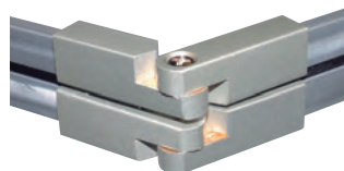
CRS355 Angular Connector Conductive 60° to 300° (240° max. range). Nickel plated allen screws, includes allen wrench.
