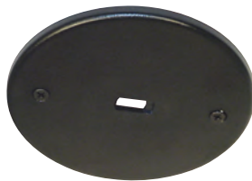
MLA-18 Mono-point, Octagon Junction Box Mount (Remote Transformer Use) Screw Holes 3-1/2" O.C.; 1/4"H x 4-7/8" Dia. Finish: - B, P, S
