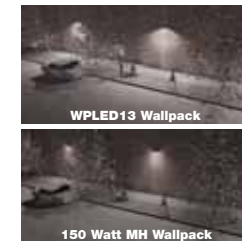
150 Watt MH Wallpack Night Time Simulations Rendered using AGI32 based on IES LM-79 Testing
