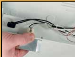
Lens and lamp assembly is easily removed for servicing.
