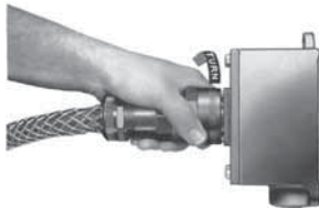
A. Turn plug clamping nut counterclockwise 45° to unlock plug.
