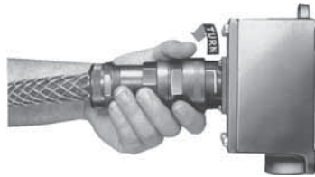
C. Turn plug clamping nut an additional 45° counterclockwise to the release position, thereby effecting delayed action.
