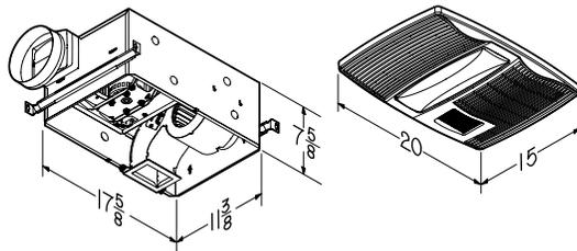
PowerHeat™ is a NuTone design that maximizes heat output per watt. With the heater element close to the forced air exit grille, the internal components are not heated. Heat is delivered into the room and does not escape into the ceiling or attic space.
