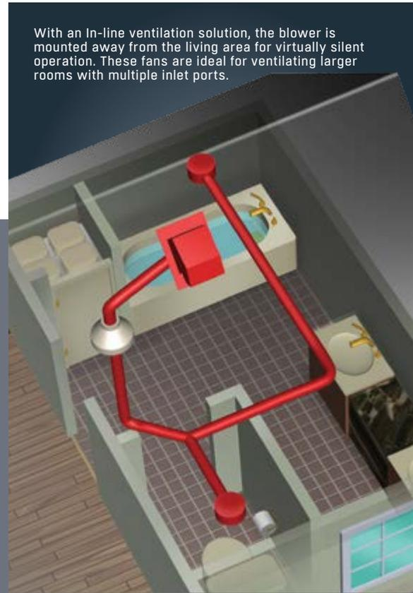
With an In-line ventilation solution, the blower is mounted away from the living area for virtually silent operation. These fans are ideal for ventilating larger rooms with multiple inlet ports.
