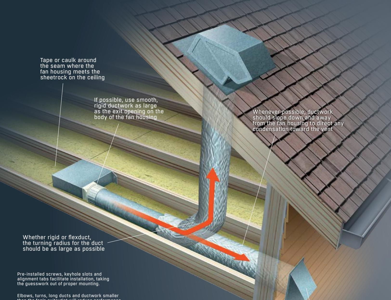
Tape or caulk around the seam where the fan housing meets the sheetrock on the ceiling
