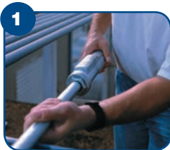
Slide the fitting onto the conduit until it stops at the internal sliding bushing. Tighten and you're ready. No parts to reassemble!
