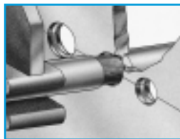
Die-type blades incorporate a counter-bored hole to the insulation and an inner cutting hole sized to the conductor. This varies depending on insulation type and thickness.
