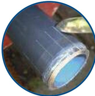
To prevent clogging, use a knife and score the conduit lengthwise from the point where the threads will end to where they begin. This will allow the PVC and metal shavings to fall into the throat of the die head.
