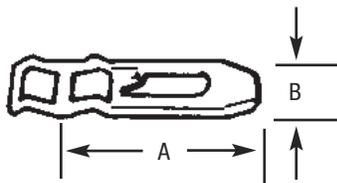
Corrosion resistant PVC coated malleable iron. Pre-mountable, stackable to eliminate offsetting.
