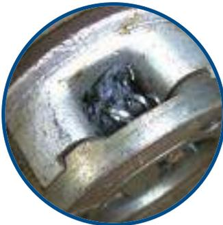
The die teeth are cutting tapered threads and will become clogged with PVC and metal shavings.
