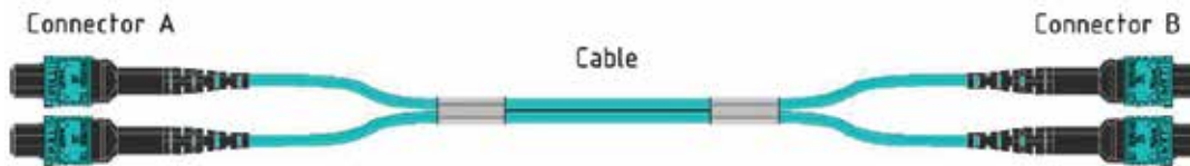
Figure 2 MPO to MPO assembly on 24 fiber 3 mm interconnect zipcord cable.
