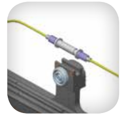
Complete Second Buffer Crimp and Remove Splice from Tool
