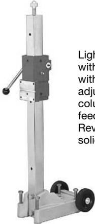
Lightweight, portable coring stand for the contractor with heavyweight applications. Cast aluminum base with 4 leveling screws for fast accurate leveling adjustment. Durable, precision-ground 2-1/2" steel column, 43-1/2" high. Rear mounted rack and pinion feed. Jackscrew for ceiling and backwall bracing. Reversible feed handle. Locking carriage. Heavy-duty, solid rubber 5" wheels. Universal motor adapter plate.
