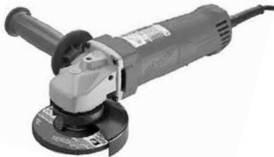
Powerful 8.5 amp motor with long life brushes and high output fans. Paddle switch with integrated lock-off button. Optimum speed for various accessories. Cast aluminum gear housing with recessed spindle lock. 3-position large flanged side handle. Adjustable wheel guard. Lock-on button for continuous operation.
