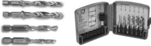
Complete hole drilling, tapping and deburring/countersinking in one operation with power drill. Back tapered beyond tap to prevent thread damage from over-drilling. Made from hardened high-speed steel for longer life. Designed to tap up to 10-gauge metal.
