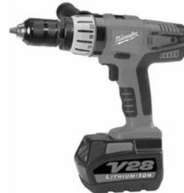
Ratcheting, single-sleeve chuck with carbide jaws for superior gripping strength. 2-speed gear box with all metal gears, delivers 0-600/0-1,800 RPM; 0-9,000/0-27,000 BPM. Clip-Lok secures tool to belt with one hand. Reversible battery pack allows user to change drill balance for overhead work on in confined areas.
