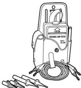
Test ALL gas-filled lamps (fluorescent, high & low pressure sodium, neon, mercury vapor, metal halide). Test fluorescent bulbs in sockets to determine bulb or ballast problem. Identifies problems with: ballasts, ignitors, starters, capacitors and resistors.
