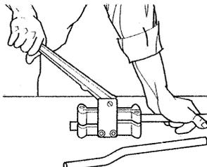
Little Kickers make offsets in 1/2" and 3/4" thin-wall (EMT) conduit in 2 seconds. Every bend is identical, no time spent refitting or cutting and trying.
