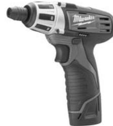
Quick bit-loading 1/4" hex chuck for bit insertion and release with one hand. Battery fuel gauge displaying remaining run-time. Metal gear housing for job site durability. Built-in LED for illumination of dark work spots. Variable speed trigger for output power control. Over-mold side and grip for secure grip and work surface protection. 0-500 RPM no load speed. 100 in.-lbs torque.
