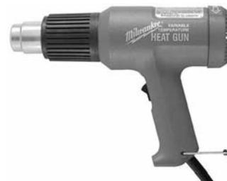
Variable temperature – 140° to 1040° F. Three position rocker switch – off, high & low. Impact resistant heating element. Efficient soft air velocity. Cool air inlet design. Support stand included.
