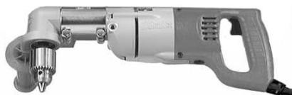
1/2" trigger speed control reversing. Helical cut, heat treated gears. Durable, glass reinforced nylon handles. Variable speed, control reversing. All ball and roller bearings. Use with up to 4-5/8" selffeed bits. Steel hardened shafts. Head and handle swivel 360° - can be locked tight in any position.
