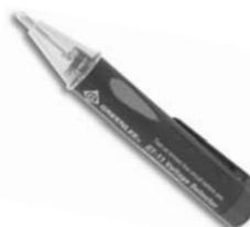
Fast, easy, non-contact voltage detection. Bright LED and audible alarm if voltage is present. ON/OFF switch for longer battery life. Use to detect the presence of voltage at outlets, lighting fixtures, circuit breakers, wires and cables or to find a break in a wire.
