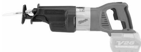
28V power at 18V battery weight. 1-1/8" stroke, 0/2,000 - 0/3,000 SPM. Tool free adjustment shoe. Exclusive gear protecting clutch for long life. Two-finger variable speed trigger.
