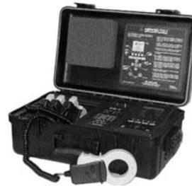
AC current up to 1000A, AC voltage, active, reactive and apparent power, energy, peak demand & power factor. All readings are true RMS. Five built-in selectable languages: English, French, Italian, German and Spanish. User selectable rates allow recording from one hour to several months. Works with single and three phase systems (Y and Delta). Readings on the DM-II LCD screen or downloaded to a PC. Capable of recording all parameters simultaneously.
