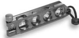
Mini torpedo design with handy "no-dog" attachment for bending. Three rare-earth magnets provide superior holding strength. Four vial design - 0°, 90°, 45°, and 30°.
