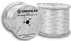
Printed sequential footage markings for accurate measurements. Durable and stretch resistant. Pre-lubricated to reduce burn-through in inner duct. Strong - 1800 lb. tensile strength.
