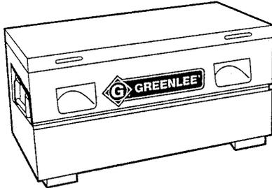
Steel support arms to hold lid in upright position. Heavy-duty piano hinges with non-removable pins. Built-in pretapped skids for easy caster installation. Dual recessed and concealed lock protectors for maximum security against drilling or cutting lock.
