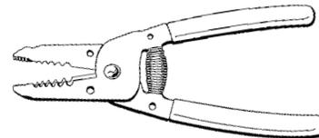
Strips six standard wire sizes: No. 10 through 20 AWG. Scissors action of 1/2" wide cutter makes clean cuts. Serrated nose jaws to bend, shape, or pull wire; holes for looping wire ends. Coil spring. Blue plastic-dipped handles.
