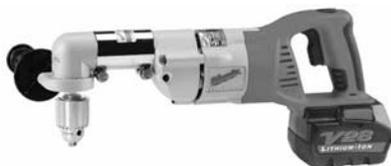
0-400/0-1000 RPM. 1/2" keyed chuck. Head swivels 360° and can be locked tight in any position. Convenient, easy reach forward/reverse lever. 28V power at 18V battery weight.
