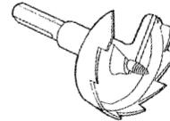
All sizes have removable and replaceable feed screws. Two feed screws furnished with each bit. Coarse feed screw provides fast, effortless feeding even in gummy woods. Inside cutting plane shaves hole radius for clean, smooth holes without pressure.
