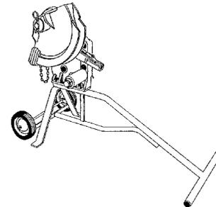
Bend 1/2" thru 2" EMT, 2" aluminum rigid, 1/2" - 1-1/2" IMC, rigid steel, and PVC coated steel conduit.
