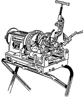
Light compact design. Threads 1/2" thru 2". Standard equipment includes: Power Drive, Universal Die Head and Dies, No. 360 Cutter, No. 344 Reamer, one gallon Nu-Clear Thread Cutting Oil and Folding Stand. Includes self contained oil system.
