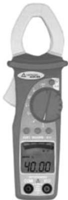
TRMS measurement. Dual displays - permits simultaneous reading of amperage and voltage. Micro Amps measurement for testing "flame sensors." Capacitance to 3000  $\mu$ f. Temperature w/Type-K thermocouple. AC and DC voltage to 600V. AC current to 400A. Resistance to 40M $\Omega$ .
