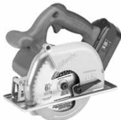
18V, 2.4 amp-hr. battery delivers long run time. One-hour NiCd charger. Electric brake for quick blade stops. Powerful motor with replaceable brushes. 3200 RPM for fast cutting. Ergonomic cushion grip D-handle. All-metal upper and lower guards.
