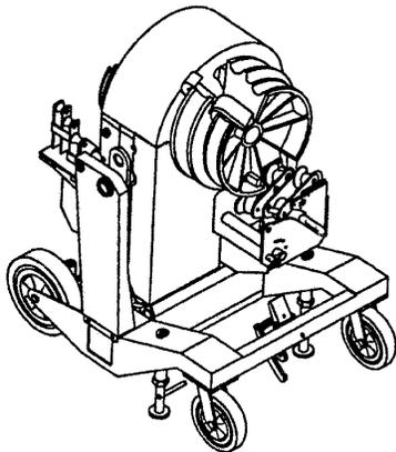
Permanently mounted bending shoes to bend EMT, IMC and rigid in sizes 1/2" to 2". Two operating positions, upright and tabletop. Intelligent pendant control, with digital readout and programmable bend angles. Built-in bending accuracy with soft stop operation, automatic springback compensation and automatic zero set.
