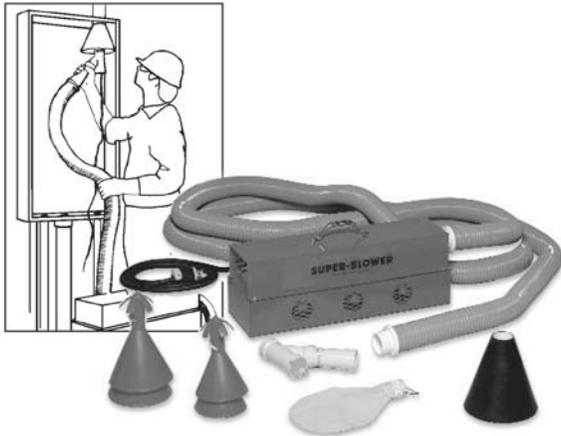
Designed for 1/2" to 6" conduit. Will blow 1/2" diameter pull rope 1,000 feet or more. 115 volt, 23 amp motor.
