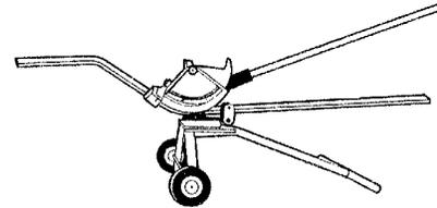
Economically bends small-diameter conduit or pipe. Ratchet action permits short, powerful strokes for easier bending. Roller support relieves friction and speeds bending. Built-in bending gauge reads 0° to 90°. Benders have "swing-away" pipe clamping device for fast loading and unloading.
