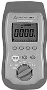
Tests insulation of wires, cables, transformers and motors. Comes as a complete kit including test leads & PC software. Three selectable test voltages up to 1000V. Built in voltmeter. Sensitive Ohmmeter for checking resistance of motor windings. Programmable timer to perform the Dielectric Absorption Ratio Test. Internal memory, 99 data-points. Data download to PC.
