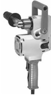
Functional design puts force in line with chuck. Power and torque, reversing, compact design for drilling between studs and joists. 2-position pipe handle. 3-position spade handle. 2-speed gear shift. External brush caps. Heat treated cut steel gears. All ball and roller bearings. Can power up to 4-5/8" selffeed bit in low speed and drill up to 1-3/8" selffeed bit in high speed.
