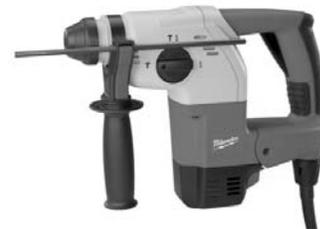
3-modes of operation; hammer-drill, drill, chipping for maximum versatility. Compact and lightweight, L-shape design. Anti-vibration, soft grip handle and two-finger trigger. 7.0 amp motor, 2.0 ft.-lbs. of impact energy, 0-5,980 BPM and 0-1,400 RPM for fast drilling and powerful chipping. Integral clutch minimizes torque reactions and helps protect gears. Heavy-duty 10 ft. Quick-Lok rubber power cord. Keyless SDS chuck for fast, tool gree bit changes.
