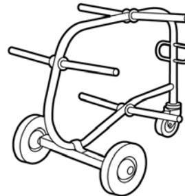
Handles six 2500 foot spools up to 18" diameter. Passes through a 30" doorway. Spindle design permits easy payout of wire with automatic braking. Front wheel is swivel mounted to permit feeding in any direction from a central location, and can be locked to resist movement.
