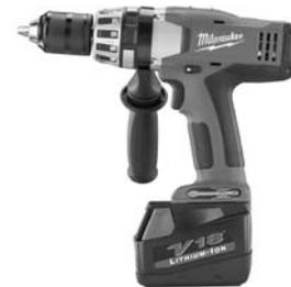
1/2" metal ratcheting chuck with carbide jaws for superior gripping strength. 2-speed gear box with all metal gears, delivers 0-450/0-1,700 RPM; 0-7,200/0-27,200 BPM. High power motor delivers 550 in-lbs of torque. Reversible battery pack allows user to change drill balance for overhead work on in confined areas.
