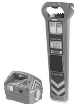
Depth measurement up to 10 ft. Precise pinpointing of buried services, exceptionally fast sound & meter response. patented Signal Processing – operates effectively in congested sites and sites with overhead cables. Locates underground energized and de-energized wires, cables and pipes. Complete instrument, ready for use with receiver, transmitter, connection cable, ground stake and ground cable. Visual (LCD) & audible indicators.
