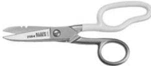
Stainless steel maintains blade durability and sharpness. Serrated teeth allow for non-slip cutting action. Free-fall snip feature for ease of use. Cuts electrical communication 19 AWG and 23 AWG wire. Extended handle provides comfort and cutting leverage for wire cutting application.
