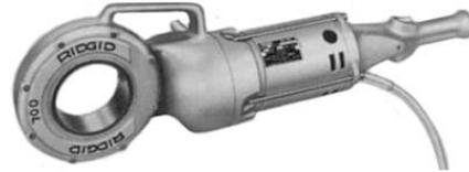
The Ridgid No. 700 Power Drive has power to cut threads and drive geared threaders. Reversible motor and all-spur gear reduction assures maximum power and efficiency. Ridgid No. 12-R die heads fit without an adapter while only four adapters are needed for other Ridgid die heads. A square drive adapter is used for Ridgid geared threaders. 1/2 HP, 115 volts.
