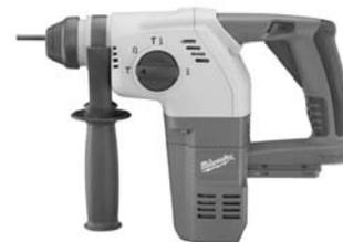
Reversible motor delivers 4,7000 BPM and 2.1 ft.-lbs. of impact energy. Optimal drilling range in concrete is from 3/16" to 3/4" with a 1" solid bit capacity and 2-1/2" thin wall core bit capacity. Three operating modes - hammer drill, drill only, and chipping. Soft-grip handle and two-finger reversible trigger for maximum comfort.
