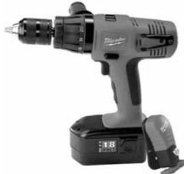
Powerful 18V motor delivers 495 in.-lbs. maximum torque. 1/2" metal ratcheting chuck with carbide jaws for superior grip strength. One-hour NiCd charger. Reversible battery pack fits into tight work spaces and adjusts balance. Two speed ranges: 0-500 and 0-1700 RPM.
