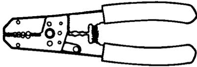
Strips 6-16 solid and 8-18 stranded and crimps terminals for 10-22 wire sizes. Cuts common sizes of bolts and screws. Has built-in wire cutter, looping holes, conduit reamer and cushioned yellow plastic grips.
