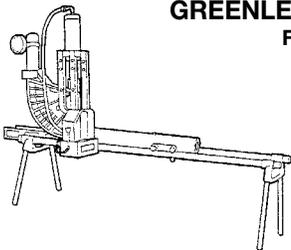
Converts Greenlee 881 bender into a comfortable, bench-high machine, makes loading faster and easier. Offset and one-shot bends in all four types of conduit. No Wows or Dog Legs. Pipe vise holds conduit and pipe securely for accurate bends. Easy to move and store. Parts stored in compact 31" x 18" x 14" metal storage box.
