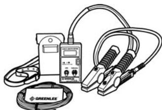
Measures the lengths of copper or aluminum wire, while still on the reel. For #10, #8, #6, #4, #2, 1/0, 2/0, 3/0, 4/0, 250 MCM, 300 MCM, 350 MCM and 500 MCM. Complete with leather carrying case, extra large clamps and calibration coil. Uses two 9 volt alkaline batteries, included.
