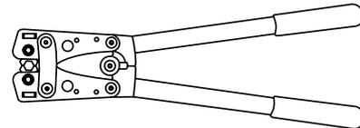
Rotatable die wheel is color coded and stamped with conductor size. Crimps lugs and splices #8 - 4/0 copper. Comfort grip handles. Heat treated steel jaws. Approximately 9000 crimp cycle life.
