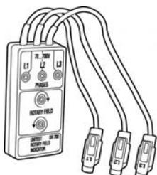
Indicates phase sequence/rotary field from 70 to 700 volts. Lights show which phase is lost. Insulated alligator clips for personal safety. No batteries or moving parts.
