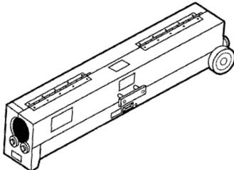
Heavy duty insulated walls and lid. Sturdy 6" wheels for easy mobility. 52" long. 115 volt, 20 amp power required. Heats 50 ft. long section of pipe.
