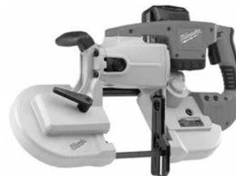
Over 200 cuts of 1" conduit per battery charge. High/low speed selector switch with lock. Two-finger trigger speed control. Comfortable non-slip soft-grip. LED light aids cutting visibility. Deep cut, full 4-3/4" x 4-3/4" cutting capacity.
