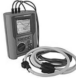
The DM-III Multitest F is a multitasking device. Measures and records three phase: voltage, current, voltage anomalies (sags or surges), harmonics energy and power (active, reactive and apparent), power factor (true and displacement), frequency and phase sequence. It can test wires and motors for proper insulation, as well as it can measure the resistance of the grounding systems and resistivity of the soil. On board memory makes it a perfect tool for preventive maintenance applications.
