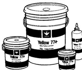
Features Teflon for added lubricity to ease installation. Stable from 30°F up to 190°F allowing use even in very hot conditions. Can safely be used with all jacket and insulation types. Dries slowly to thin, soft, non-conducting film that won't harden in conduit. Will never require the use of cable removal chemicals. Non-toxic, non-flammable, non-combustible, and non-corrosive.
