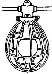
For temporary jobsite lighting. 100 ft.; 10 medium base sockets and yellow plastic guard assemblies at 10 ft. intervals, two 14-gauge wires. 1500 watt capacity. Bulbs not included.
