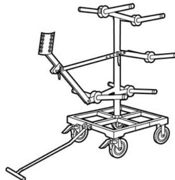
Holds ten 2500 foot spools from No. 22 to No. 10 wire, up to 18" diameter spools. Passes through a 36" doorway. Spool rack and guide head rotates 360°. Guide head can be raised or lowered approximately 30%. Large 8" casters, 2 lockable. Guide head gathers and straightens the wire for easy feeding. Eliminates kinks or tangles.
