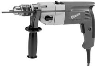
For percussion drilling with carbide-tipped hammer-drill bits in concrete and masonry or drilling without hammering in wood or metal. Trigger speed control. 1/2" keyed chuck. All ball and roller bearings. Side handle can be used on either side and with or without depth gauge. Self-stopping brushes. Soft grip handle. Heavy-duty metal gear case for rugged durability. 10 ft. Quik-Lok cord.
