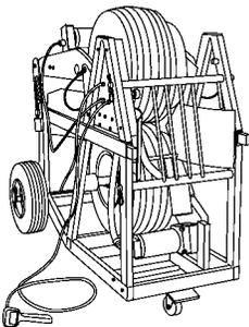
Feeds cable at variable speeds to match the speed of cable puller. Accommodates cable ranging in size up to 3.5" in diameter. Sets up easily and can be operated by just one person. Dual motors drive each wheel for traction on both sides of the cable.
