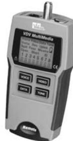
Easy-to-use tester for installers working with voice, data, and video applications. One tester for all applications. **Voice:** Supports 3-pair USOC and 6-position RJ-11/12 jacks for telephone cable testing. **Data:** Supports both shielded and unshielded cable testing to T568A/B (RJ-45). **Video:** Tests coax cable for opens and shorts with F-connector interface.
