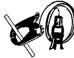
For use with any Amprobe clamp-on AC ammeter (including certain recorders and multimeters) to extend current ranges by 10 times up to 1200 amps intermittent duty (20 seconds maximum), 600 amp continuous duty. Instrument clamps around pick-up coil at end of line cord, which is 2 feet long for remote readings. Accommodates cable up to 2" in diameter or 2000 MCM, and bus bar 3/4" x 2-1/2". Insulated for use on circuits up to 3300 volts, 4200 volts peak.
