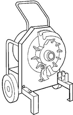
Bends 1/2" thru 2" rigid, EMT, or IMC with proper bending shoes. Makes 90° bends in 2" conduit in 16 seconds, 1/2" to 1" in 10 seconds. Simple set up and easy operation for correct bends every time. Squeeze adjustment on roller support accommodates variations in conduit. Easily portable...fits thru a 30" opening. Skid type handles permit horizontal bending for larger offsets and saddles. Makes 180° bends in one setting on 1/2" thru 2" rigid conduit.
