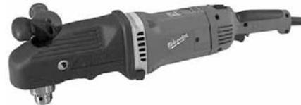
Highest amp rating (13.0) and power-to-weight ration in its class. Low speed clutch protects gear train. Fast drilling - highest RPM in its class. Maximum SFB at 1., 750 RPM - 2-9/16". Maximum SFB at 450 RMP - 4-5/8". Roto-Lok rotating handle - 90° left/right rotation for most comfortable grip position. T-bar front grip helps guide bit. cushion grips provide more comfortable gripping. Efficient gear shift design.
