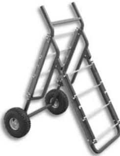
Holds up to twenty four (24) spools of #12 AWG wire or sixteen (16) spools of #10 AWG. Folds for easy storage. 10" diameter pneumatic tires for jobsite portability.
