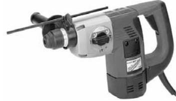
D-style handle offers a secure grip that maximizes drilling pressure while minimizing operator fatigue. Electronic variable speed control trigger. 3-modes of operation; hammer-drill, drill only, and chipping for maximum versatility. Chisel adjustment allows bit to be position to the workplace to maintain comfortable tool orientation while chipping. Slip clutch stops action when jammed.
