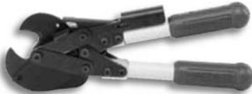
Two-speed mechanism saves cutting time by closing the blades rapidly and shifting to normal speed to perform the cut. No more pushing on stubborn release button—the blades open automatically when the cut is complete. Completely new ratchet mechanism improves durability.
