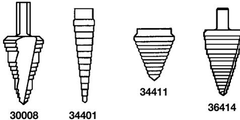
Drills steel, brass, copper, aluminum, wood, and plastics. Model 34411 drills a perfect KO for 1/2" conduit (7/8"); model 36414 drills both a 1/2" KO (7/8") and a 3/4" KO (1-1/8").
