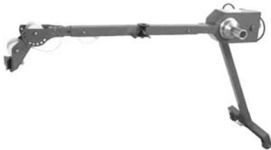
Quick latch system attaches to all conduit sizes with no loose parts. Adjustable elbow and extendable boom adjust easily. Right angle sheave keeps operator out of direct line with pulling ropes. Two pulling speeds.
