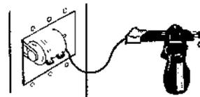
Increase the current measuring sensitivity of Amprobe clamp-on ammeters, recorders, and multimeters by 10 times for more precise current readings on small appliances and fractional horsepower motors. Effectively "splits" two-conductor line cord for reading at outlets under load. Permits voltage measurement at outlet under actual conditions. Capacity: 15 amps, continuous duty; 16 to 20 amps, one minute. Supplied with model T carrying case.
