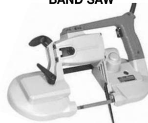
Powerful motor with long life brushes and high output fans. Optimum speed range - cuts pipes, bolts, re-bar, angle iron, tracks and other profiles in a variety of materials. Includes Super-tough Bi-Metal blades. Use standard 44-7/8" x 1/2" .020" band saw blades. All ball and roller bearings. High torque worm gear and chain drive mechanism. Excellent balance. Open line of sight for more accurate cut. Blade tightening lever.
