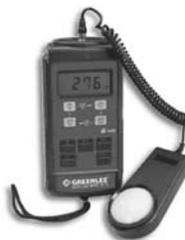
Measures incandescent, fluorescent, metal halide, high-pressure sodium and halogen lamp output. Color and cosine-corrected for enhanced accuracy. Measure up to 50,000 lux.
