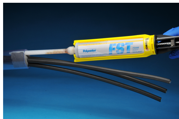
The FST™ Sealant comes in a caulking style (one plunger) tube. Package allows multiple seals. Mixing is done in the nozzle as the sealant is injected.
