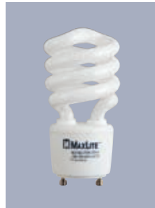
MLS13GUWW-128 13w self-ballasted lamp. GU24 base.
