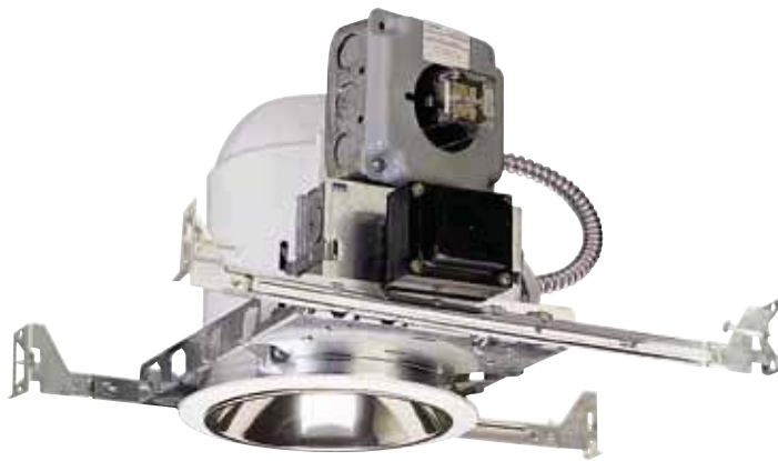
NL-601/EM 6" 12V MR16 Emergency Housing, 50W
