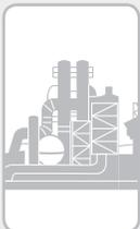
**DIVISION 1** designates an environment where ignitable concentrations of flammable gases, liquids, vapors or dusts can exist some of the time or all of the time under normal operating conditions, or where easily ignitable fibers and flyings are manufactured, handled or used.
