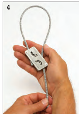
4 Push wire rope through clamp leaving 2" to 3" tail, then apply tension on wire rope
