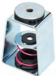
CH30SCS Type Deflection Combination Hanger 15° Tilt Spring & Neoprene w/ Seismic Cushion Stop 1" & 2" Deflection Pages 272 - 273
