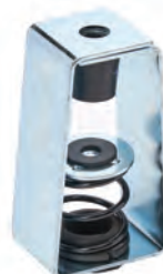
HH30SCS Type Deflection Combination Hanger 15° Tilt Spring & Neoprene w/ Seismic Cushion Stop 1 1/2" & 2 1/2" Deflection Pages 276 - 277
