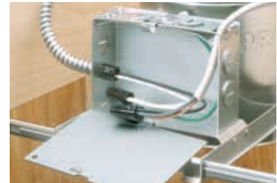
Large junction box provides four Romex and five conduit knockouts. Listed for through-branch circuit conductors. Cover is hinged to prevent accidental loss.
