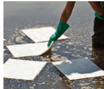
Clean up oil and petroleum-based spills on land or water with specialized sorbents that don't absorb water.
