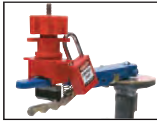
Clamp attaches to butterfly handles, preventing trigger handle from being squeezed. Valve cannot be repositioned!
