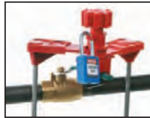
Use two blocking arms to lock out 3-, 4- or 5-way valves, or to lock valves in the "on", "off", or "throttled" position for operational control.
