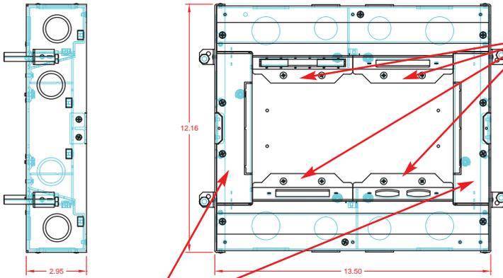
**MAIN** compartment areas include two duplex, two Decora and one 6-IPS brackets. Additional brackets are available as an option. (See ordering table)
