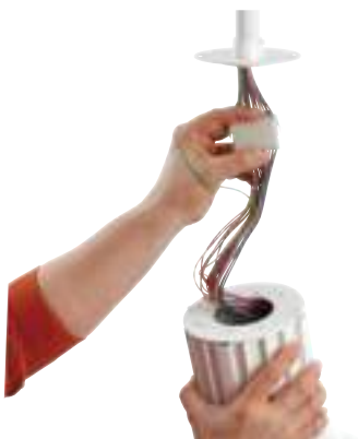
Multi-Lamp Plug & Play: 1: Install stem 2: Attach luminaire top plate 3: Plug color coded harness into the ballast 4: Plug in the luminaire
