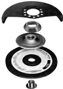
GUARD SETUP FOR TYPE 27 WHEELS WITHOUT THREADED HUB
