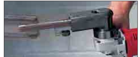
Grind and deburr ends of metal stock.
