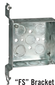
"FS" Bracket Mounts on flat side of stud. Gauging tabs and recessed nailing spurs.
