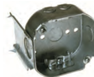
"J" Bracket Spurs, slotted holes for toe-nailing. Gauging notches at 3/8" and 1/2".
