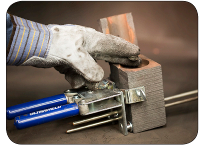
Step 3: Insert disk into mold.
