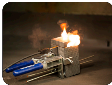
Step 5: Reaction is made, open mold to remove connection and clean mold before next connection.
