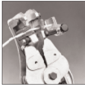
Transparent wire stop provides uniform stripping length.
