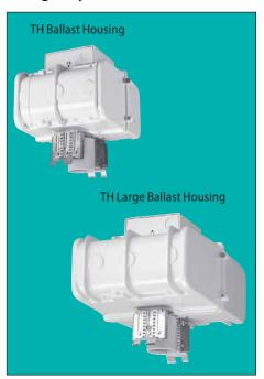
Modular ballast housing for high bay opticals. Pre-attached adjustable legs accept a wide selection of anodized aluminum and prismatic acrylic high bay reflectors. A variety of distribution patterns at higher mounting heights can be achieved. These systems
