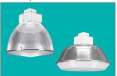
Low bays are designed with distributions to spread the light out in a space and prevent hot spots of light below the luminaire. The bottom prismatic lens bends the light to create wide distributions that improve uniformity and increase vertical illumination at lower mounting heights. Low bays perform best at mounting heights less than 20 feet and are available in various wattages up to 450 watts. The prisms reduce glare and
