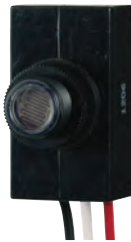
80-1733 Photoelectric Switch Plastic DOS Shell, Rated: 500W-120V For Outdoor Use-Incandescent 2" H x 1 1/8" W x 7/8" D
