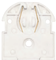
80-1249 Butt-On Mounting T8 or T12 Lampholder Rapid Start Applications 1 7/16" H x 1 3/8" W x 3/8" Dia. 660W-600V
