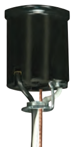
80-2036 Medium Base w/Rim 1/8 IP Hickey 12" AWM B/W 105°C Leads & Ground Wire Overall Ht. 2" Dia. 1 1/4" 660W-250V
