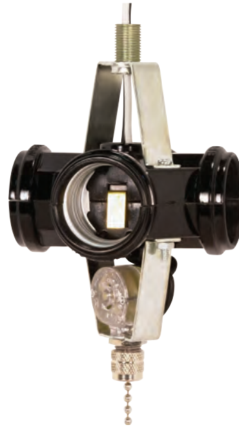
90-1588 4 Light Cluster Socket On-Off Nickel Pull Chain 1 3/4" 1/8 IP Threaded Top Bracket w/ 1/2" Nipple 1 3/4" 1/8 IP Threaded Bottom Bracket 7" AWM B/W Leads 105°C 660W-250V
