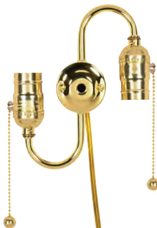
80-1268 Brite Gilt Twin Pull Chain Brite Gilt Chain and End Ball with 1/4" 18/2 SPT-2 105°C Clear Gold Wire Internal Wire - 18 AWM 105°C 7" Centers 1/8 IP Top and 1/8 IP Bottom 660W-250V
