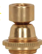
90-2593 Large Hang Straight Swivel 1/4 F Top - 1/8 F Bottom Ring Nut to Seat 1 1/16" 1 1/2" Height Unfinished
