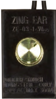
80-1166 Full Range Table Lamp Dimmer Switch Phenolic Housing Black 2" x 1 1/4" x 1 1/8" 12" AWM 105° C Black Leads Strip 1/2" w/Two Knobs: Black & Gold 300W-120V
