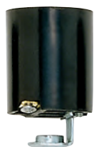
90-407 1/8 IP Hickey Screw Terminals Overall Ht. 2" Dia. 1 1/4" 660W-250V
