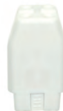
80-1490 Circle Connector-Quickwire Used with High Voltage Instant Starting Transformers Accepts 18 AWG Leads Solid or Stranded w/Brass Alloy Contact 7/8" H x 5/8" W 660W-600V
