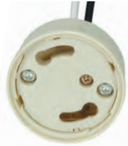
80-1859 24" 18 AWM 105° Leads 80-1935 w/Quick Wire Terminals 1/8 IP Bushing Height: 3/4"
