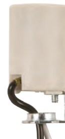
90-1555 1 3/4" x 1" W 1/8 IP Inside Extrusion 8" AWM B/W 105°C Leads Pulled Thru Single-Leg 75W-250V
