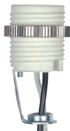
80-2543 2" Ht. - 7/8" Dia. 18" #18 UL 1015 B/W Leads 105°C w/Chrome Metal Ring 1/8 IP - Inside Extrusion Single-Leg 75W-125V
