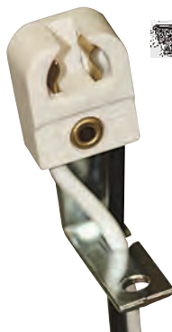
80-1251 T5 Lampholder w/8" AWM B/W Solid Leads for Retro Fit and Replacement Tall Right Angle Bracket 1 1/4" H x 5/8" W x 3/8" Dia. 660W-600V
