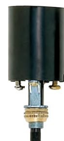
90-4300 Bottom Turn Knob Screw Terminals 1/8 IP Ht. 2 1/2" Dia. 1 1/4" 3/8" Bushing 660W-250V
