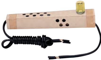
90-1082 Full Range Pole Lamp Dimmer Switch Paper Housing 4 3/4" x 3/4" 500W Pole or Post Lamp Dimmer w/One End 2 ft. Leads SPT-1 Black Other End 7" SPT-1, Strip 1/2" w/One Brass Knob 500W-120V
