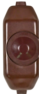
80-1481 Brown 80-1482 Ivory Full Range Lamp Cord Rotary Dimmer Switch 3" x 1 1/4" For 18GA SPT-1 or SPT-2 Wire Phenolic - 200W-120V
