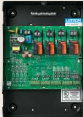
Energi Savr Node with lid removed for button-press programming
