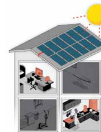
Daytime: Important loads are powered first by the PV system and then by the battery. The battery can be charged from the PV as needed
