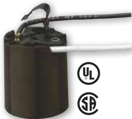
70146 Vertical Phenolic Snap-In Socket Fits into 3/8" x 1/4" Hole Medium Base 660 Watts Max. 250 Volts
