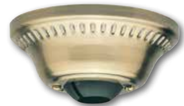
77060 - Antique Brass Finish 77061 - Polished Brass Finish 77268 - White Finish Canopy Kit 1/2" I.D. Ball Included Can be mounted onto a cathedral ceiling having up to a 25° angle 100 lb. Load Rating
