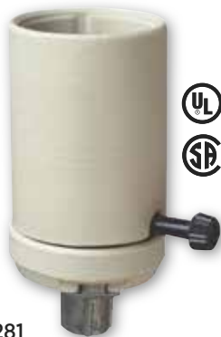
* 22281 Mogul Base Socket 3-Way Removable Knob Bushing ¼-IP 750 Watts Max., 250 Volts Height - 4¼"
