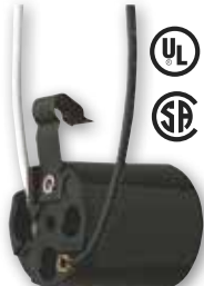
70145 Horizontal Phenolic Snap-In Socket Fits into 7/8" x 1/4" Hole Medium Base 660 Watts Max. 250 Volts
