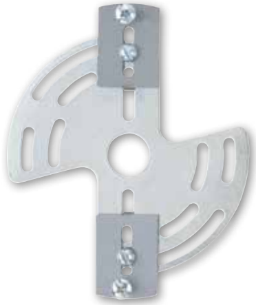
*21032 70111 Adjustable All-Purpose Crossbar Slips \frac{3}{8} -IP Holes Tapped 8-32 Adjusts from 3 \frac{3}{8} " to 5" for Slot Mounting on 3", 3 \frac{1}{4} " or 4" Box Two \frac{1}{2} " Head Screws Included Two \frac{1}{4} " Head Screws Included 35 lb. Load Rating
