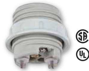
70010 Porcelain Threaded Socket with Aluminum Shade Ring Medium Base Height - 1 5/8" Ring Height - 1/2" 660 Watts Max. 250 Volts
