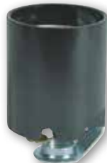
70407 Keyless Phenolic Socket 1/8-IP Hickey Medium Base 660 Watts Max. 250 Volts
