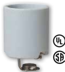
* 22267 Keyless Socket Medium Base 1/8-IP Hickey 660 Watts Max. 250 Volts Height - 2" 1875 Pulse Rated
