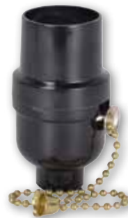
70433 Pull Chain Phenolic Socket On/Off Tapped 1/8-IP Medium Base 250 Watts Max. 250 Volts
