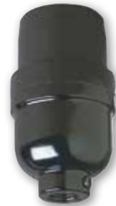
* 22234 High Heat Phenolic On/Off Medium Base Keyless Bushing 1/8-IP with Set Screw 660 Watts Max. 250 Volts Height - 2 3/4"
