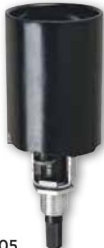
* 22205 1-Piece Phenolic Shell Bottom Turn Knob Socket Medium Base Nipple 1/8-IP 660 Watts Max. 250 Volts Height - 3 1/4"
