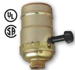
* 22051 - Polished Brass 2 Circuit Turn-Knob Socket Medium Base Bushings 1/8-IP with Set Screw Removable Knob 250 Watts Max., 250 Volts Height - 2 1/2"
