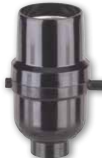
* 22237 Push-Through Phenolic Medium Base 1/8-IP Cap with Side Screw Aluminum Screw Shell 660 Watts Max. 250 Volts Height - 2 5/8"
