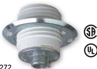
*22272 70429 Porcelain Threaded Socket with Steel Shade Ring Medium Base Bushing 1/8-IP with Set Screw Height - 2 1/8" Ring Size - 2 1/4" 660 Watts Max. 250 Volts
