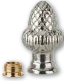
70141 Acorn Knob Lamp Finial Nickel Finish Height - 1½" Tapped ¼-27 Finial Thread Reducer Tapped ⅛-M to ¼-27-F
