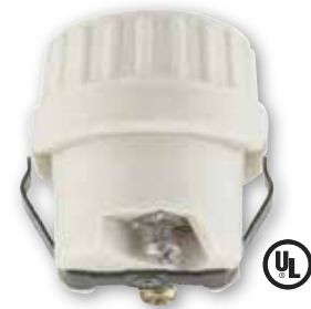
* 22276 Snap-In Porcelain Socket Medium Base 660 Watts Max., 250 Volts Height - 1¾"
