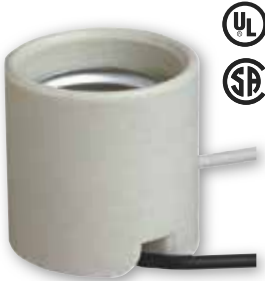
* 22218 Keyless Socket One Screw Surface Mount Medium Base 7" Wire Leads 660 Watts Max., 250 Volts 105° Leads Leads Height - 1½"
