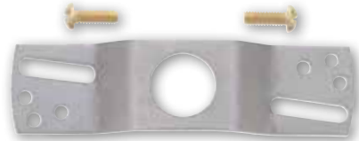
70112 4" Offset Crossbar Two \frac{1}{2} " Mounting Screws and Two Tapped \frac{5}{32} Holes Spaced 2 \frac{3}{4} " Apart Slips \frac{3}{8} -IP 35 lb. Load Rating
