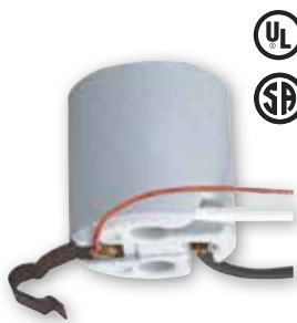
* 22372 Snap-In Porcelain Socket Medium Base 9" Wire Leads Fits ¾" x ¼" Hole 18 Gauge, 105° Leads 660 Watts Max., 250 Volts Height - 2"
