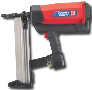
Trak-It C4 EX is a gas-powered fastening system used for light-duty static applications including drywall track to concrete, block or steel, wire lath to concrete or block, furring strips to concrete or block and plywood to concrete and block base materials.
