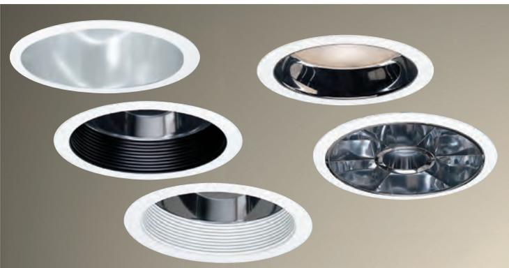
**Reflectors** PDS offers a full range of reflector options including open, open wall wash, baffle and lens with a choice of patterns. One-piece construction avoids internal losses and light leaks that occur at the ceiling line. PDS provides a 5/8" overlapped flange to cover the ceiling cutout and provide a gap free aperture with no light leaks around the flange or visible cut edge of ceiling tile.
