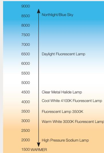
a lower color temperature than a blue white light. Psychologically, the lower Kelvin temperatures are perceived as “warm”, the higher as “cool”, the opposite of what might be expected. With discharge sources such as compact fluorescent and HID light is produced by methods other than heating a filament and the color is measured by its correlated color temperature (CCT). It is the measure of the color of the light, not the actual operating temperature of the lamp.
