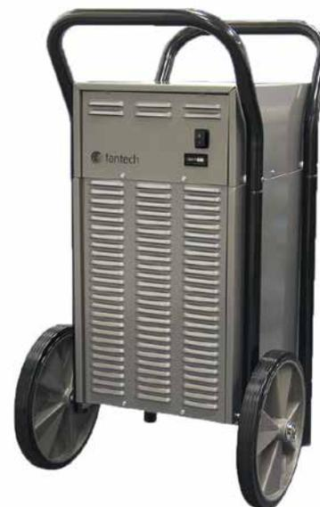
**Light Duty GD55S model** provides up to 325 cfm with 2-speed fan. Includes a dehumidistat and overflow protection with an indicator light. The steel cabinet is painted black. Equipped with fold'down handle and 4 casters.
