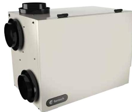
During the defrost sequence, a motorized damper temporarily blocks the incoming fresh air stream so that the warm air from the house can circulate through the HRV. The exhaust blower shuts down and the supply blower switches into high speed to maximize the effectiveness of the defrost strategy. During this cycle, household odors from the kitchen or bathroom are prevented from entering the home and the unit will not create negative pressure.
