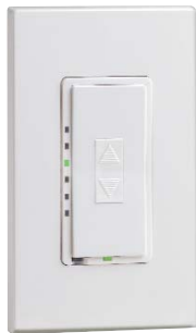
Mural L/S Preset Dimmer Decora rocker style digital dimmer with LED brightness level indicators. With inner rocker for setting brightness when lights are off. Color-change kits available. ML106-1LW shown
