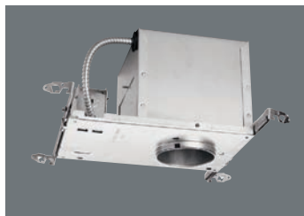
P831-AT Ceiling opening: 4-1/2" Plaster frame: 8-3/8" x 13" Recessed depth: 7-1/2"
