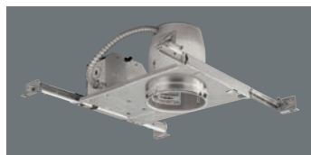
P830-TG Ceiling opening: 4-1/2" Plaster frame: 7-7/8" x 10-3/4" Recessed depth: 5-1/2" Pryouts: 1/2" and 3/4"
