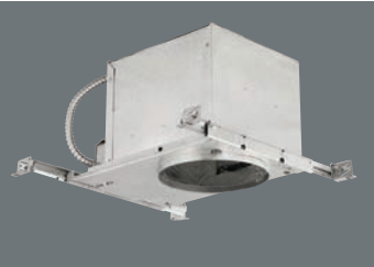
P645-TG Ceiling opening: 6-7/8" Plaster frame: 8-3/8" x 13" Recessed depth: 7-5/8" Pryouts: 1/2" and 3/4"
