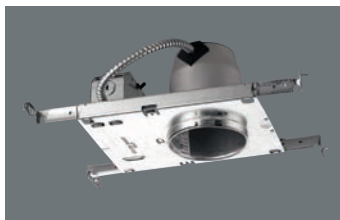
P830-18ICAT P830-13ICAT Ceiling opening: 4-1/2" Plaster frame: 17-7/8" x 10-3/4" Recessed depth: 5-1/2"
