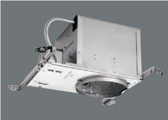
P645-AT Ceiling opening: 6-7/8" Plaster frame: 8-3/8" x 13" Recessed depth: 7-5/8" Pryouts: 1/2" and 3/4"
