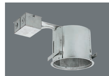
P186-TG Ceiling opening: 6-5/8" dia. Recessed depth: 5-1/2" Pryouts 1/2"
