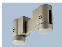
P8795-09 Brushed Nickel Illuma-Flex track link (non-powered). Mechanically joins two sections of track together. Designed to be used with or without support stem. Size: 3-3/8" W., 1-5/8" ht.
