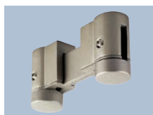
P8778-09 Brushed Nickel Illuma-Flex Power link. Electrically links two sections of track together. Designed to be used with or without support stem. Size: 3-3/8" W., 1-5/8" ht.
