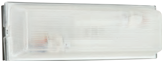
F7206-44 Fluorescent Wall Fixture 13-1/4"W - 4-1/2"H - 3-3/4"E Die-Cast Metal Housing Acrylic Lens 2-13W PL 4100K Included
