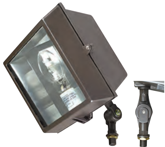
Metal Halide Flood Fixture (Large) 10"W - 10-1/2"H - 7"E Die-Cast Aluminum Housing Tempered Glass Lens Bronze Powder Coat Finish UL Listed - Wet Locations
