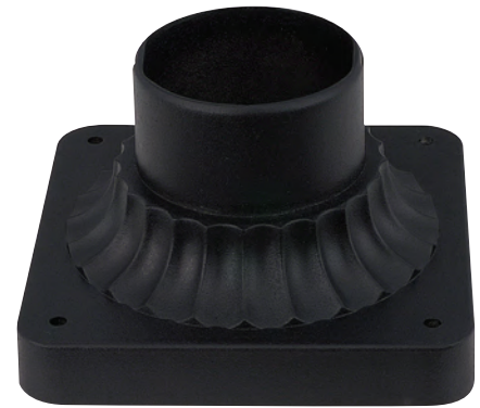
K635-30 (WH) Cast Aluminum Pier Mount K635-31 (BK) Top Outside Diameter 3" K635-62 (RB) 3-5/8" H - 5-7/8"Base Square w/4 Mounting Holes 6-3/4"C. to C. for 1/4" Screws on the diagonal
