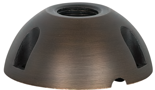
B2014 Dome Base Cast Brass Matte Bronze Finish 2.75"D Center Hole 1/2"NPT Female
