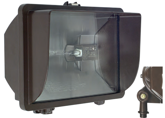
Quartz Flood Fixture w/ Glare Shield 9"W - 8"H - 5-5/8"E - 120V Die-Cast Aluminum Housing Tempered Glass Lens Bronze Powder Coat Finish UL Listed - Wet Locations
