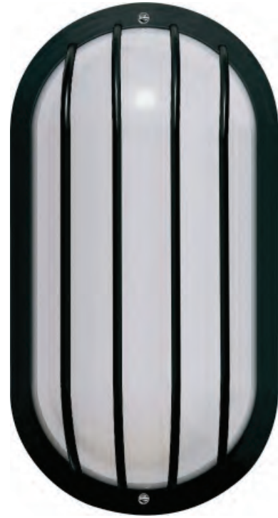
F7994-31 (BK) 5-3/4"W - 10-1/4"H - 4"E 1-13W PL 4100K Lamp (Incl) White Acrylic Lens Wet Location
