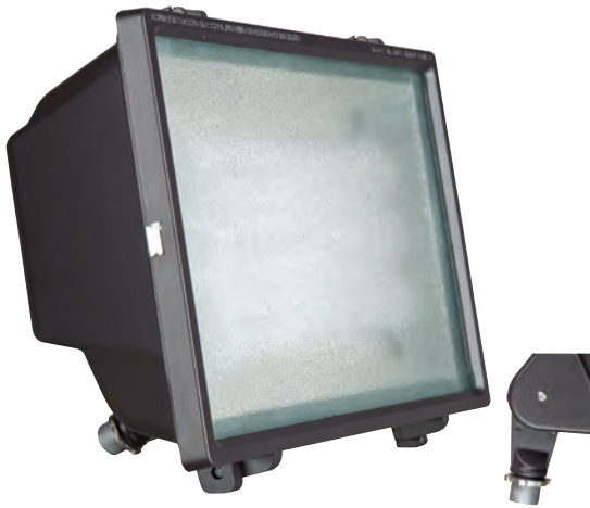
F7837-66 (BZ) Fluorescent Flood Fixture 13"W - 8-1/2"H - 4-1/2"E Die-Cast Aluminum Housing Tempered Glass Lens Bronze Powder Coat Finish 65 Watt T4 4-Pin GX-10q-4 6500K (Lamp Included)
