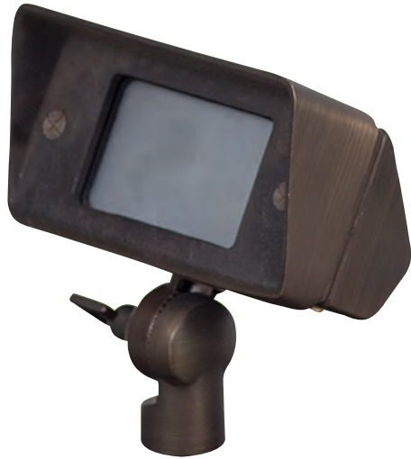
FG1552-76 (MB) Little Wash Cast Brass Directional Light Matte Bronze Finish 4"W - 4"H - 2-1/2"Depth 20W JC G-4 Halogen Bi-PIN Lamp Included Spike Included 1/2 IPS Male Thread
