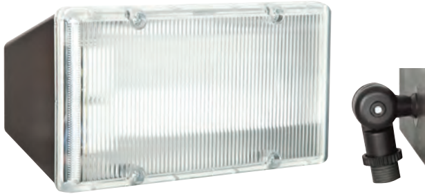
F7876-66 (BZ) Fluorescent Flood Fixture 8-1/2"W - 4-1/2"H - 4"E Polycarbonate Housing Acrylic Lens 2-13W PL 4100K Included
