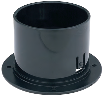
K625 Plastic Pier Mount Top Outside Diameter 3" 2-3/8"H - 4-1/8"Base 4 Mounting Holes 3-1/2"C. to C. for 1/4" Screws for direct use with Fixture Black
