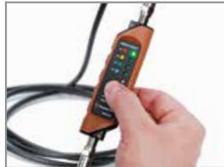
Test patch cables or installed cables
