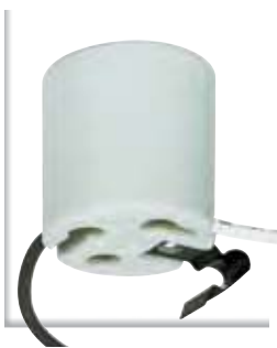
80-2652 Snap-In Socket Bracket Extends 3/8" from End of Socket 12" AWM B/W Leads 150°C 660W-250V
