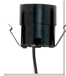
90-541 Snap-In Socket for 3 1/4" - 4" Holders 8" AWM B/W Leads 105°C 660W-250V
