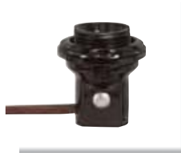
80-1473 1 1/4" with Shoulder and Phenolic Ring 24" 18/2 SPT-1 Brown Leads 105°C 75W-125V
