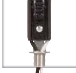
90-739 1 1/8" Smooth 6" AWM B/W Leads 105°C 1/8 IP Nipple Single Leg, 75W-125V
