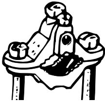
Two-screw ground connection for armored ground wire.
