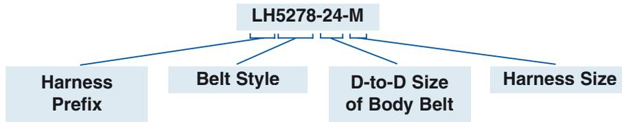
In addition to the body belt ordering procedure to determine D-to-D Size, use the following guidelines to properly identify and select the Lineman's Harness catalog number.
