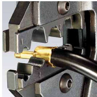
Crimp System Pliers 97 43 200 with crimping dies 97 49 35 for spark plug connectors
