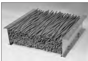
"50%" Fill Per NEC Cross Sectional Area Calculation
