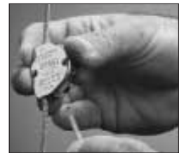
5. Thread wire rope into other side of locking device
