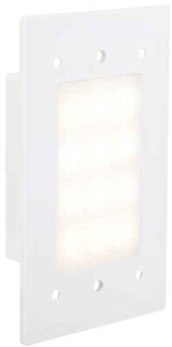
SGL-LED-WW 120-277V 1.5W / 37Lm SGL-LED-WW-12V 12V 1.5W / 37Lm Light Module - Warm White 2-3/4"W x 4-1/2"H x 1-1/2"D
