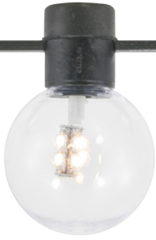
12V LED Festoon Socket Assembly 3000K / 1.5W / 80,000hr rated life Black base; max run = 300W LFS-12V-1.5-LED-WW 1.5 watts
