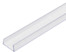
H2-TRACK-3 3ft clear plastic mounting track 23/32" w x 13/32" h
