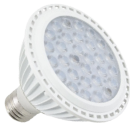
2790-12PAR30S-40-WL PAR30 40° (2700K) 12W / 830Lm / E26 75W equivalent
