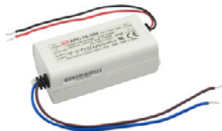
LED-DR16-350 350mA constant current hard- wire driver; Class 2, 4-16W, cURus Recognized 3-1/2"L x 1-5/8"W x 1-3/16"H
