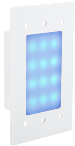
SGL-LED-BL 120-277V 1.5W / 468nm Light Module - Blue 2-3/4"W x 4-1/2"H x 1-1/2"D
