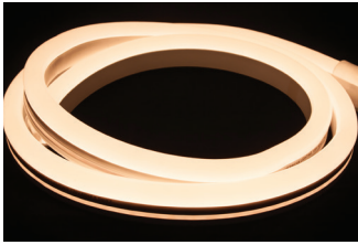
P2-NF-WW (120V) P2-NF-24V-WW (24V) Warm White LEDs • 79CRI Opaque white jacket (120V) 2700K • 63Lm/ft (24V) 2700K • 90Lm/ft
