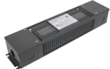
ELV-60J-24 1-60W driver ELV-80J-24 1-80W driver Class 2 dimming hardwire driver w/junction box, 60% minimum load; Dimming consumes ±3W internally
