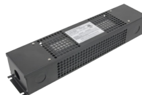
ELV-60J-24 (36-60W) ELV-80J-24 (48-80W) Class 2 dimming hardwire driver w/ junction box, 60% minimum load; Dimming consumes ±3W internally
