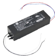
LED-DR18-350D2 350mA dimmable constant current hardwire driver with 8" lead wires; Class 2, 3-18W, cURus Recognized 5-1/4"L x 1-5/8"W x 1-1/4"H
