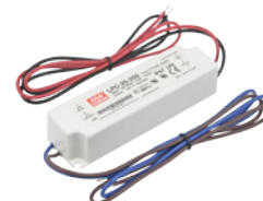
LED-DR20-350 350mA constant current hardwire driver; Class 2, 9-20W; cURus Recognized 6-5/8"L x 1-1/2"W x 1-3/16"H
