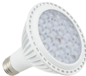
2790-12PAR30L-40-WL PAR30 40° (2700K) 12W / 830Lm / E26 75W equivalent
