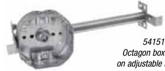
54151 AF Octagon box mounted on adjustable bar hanger. 50 lb. load max rating.
