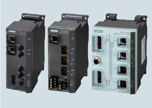
SCALANCE X-200IRT switches are especially designed for constructing isochronous real-time (IRT) Industrial Ethernet networks in line, star and ring topologies at transmission rates of 10/100 Mbit/s (Redundancy Manager integrated); construction of redundant ring connections possible.
