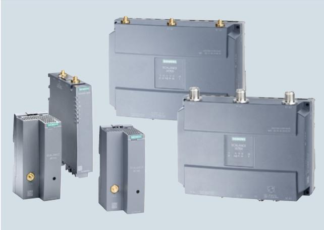
The client modules from the SCALANCE W700 product lines are optimal for integrating Industrial Ethernet stations into Industrial Wireless LANs (IWLANs) for 2.4 GHz and 5 GHz.
