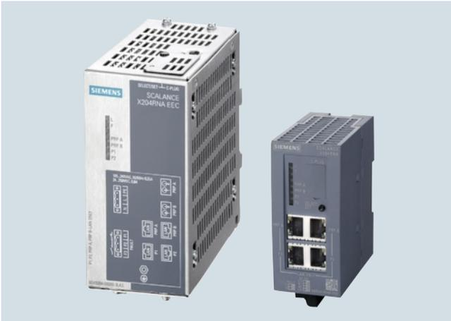
The SCALANCE X-200RNA (**R**edundant **N**etwork **A**ccess) managed Industrial Ethernet network access points with PRP functionality (**P**arallel **R**edundancy **P**rotocol in accordance with IEC 62439-3) are used to connect up to two non-PRP-enabled terminal devices or network segments to parallel networks.
